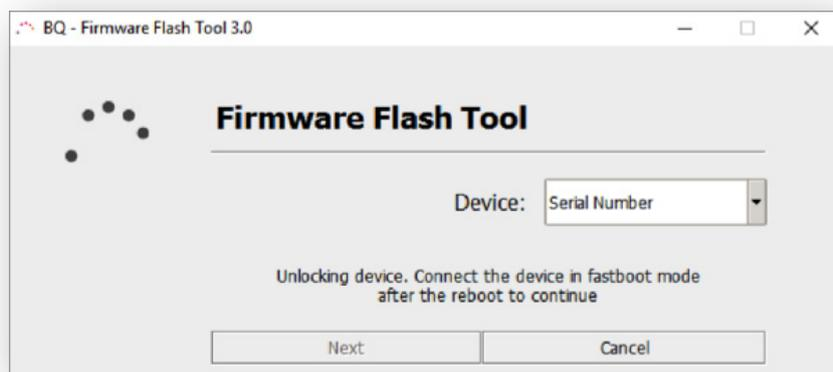
After each reboot the device remains in normal mode. Without disconnecting the smartphone from your PC, turn the smartphone off and then in FastBoot mode turn it back on (see [step 2](#)). The application detects the device again and continues the process until the unlocking process is finished.
